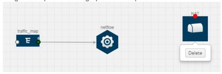
Drag and drop a link from the NetFlow application to a NAT device. A Link quick view is displayed. It is a header transformation operation that lets you configure the IPv4 destination IP of the NetFlow collector.
